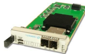
AMC626 Storage Module
